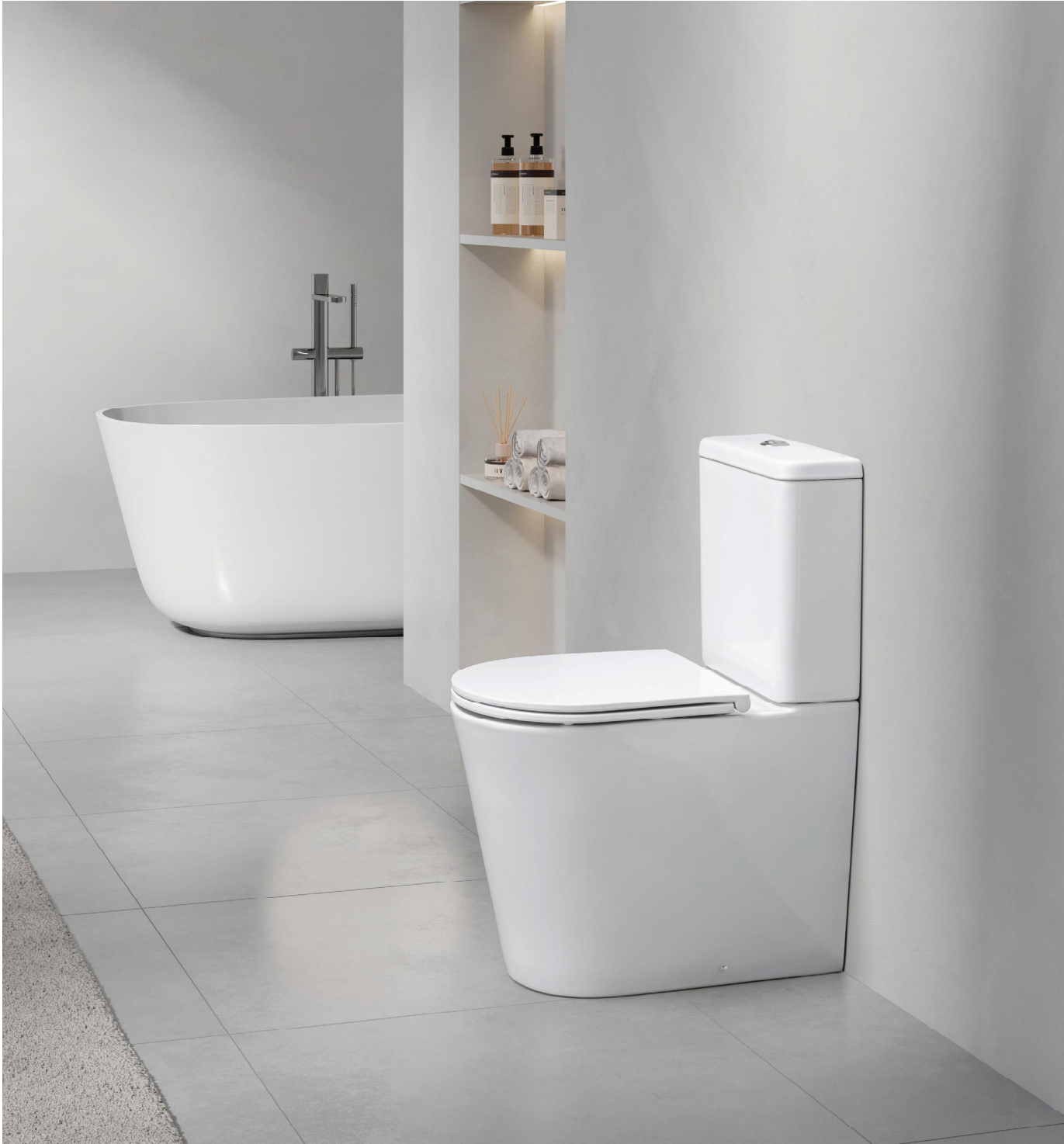
HDC821P+HDS821 Rimless Washdown Close-coupled Toilet Size 610x370x832mm P-trap P=180mm roughing-in 3/4.5L
