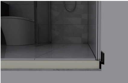
Connect method between waterproof plate and wall panel
