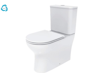
HDC836BP+HDS835A Aqua Vortex Washdown Close-coupled Toilet Size 650x375x780mm P-trap P=180mm roughing-in 2,6/4L
