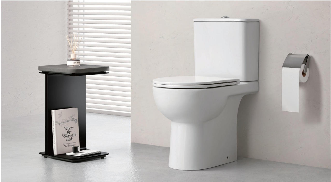
HDC835P+HDS835A Aqua Vortex Washdown Close-coupled Toilet Size 610x375x780mm P-trap P=180mm roughing-in 3/4.5L
