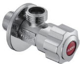
HDJ810K1 Angle valve G1/2 Brass body, ABS handwheel, chrome.
