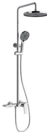
HWB5102-P01CP Shower column 3 functions, brass body, ceramic cartridge, multi-function hand shower, 10' shower head, chrome,
