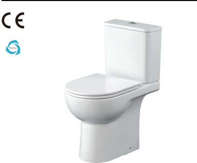
HDC835P+HDS835A Aqua Vortex Washdown Close-coupled Toilet Size 610x375x780mm P-trap P=180mm roughing-in 3/4.5L
