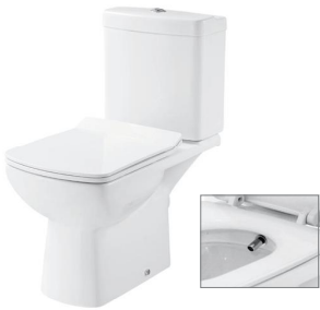
HDCB201NP+HDS201E Washdown Close-coupled Toilet Size 730x370x790mm P-trap P=180mm roughing-in 4/6L
