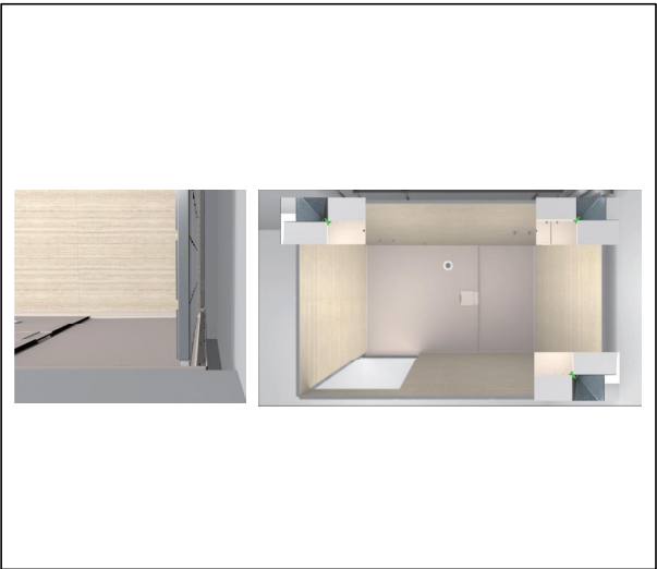
Connect method between waterproof plate and wall panel
