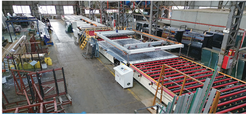
High temperature digital color-glazed glass inkjet printer 高温数码彩釉玻璃喷墨打印机
