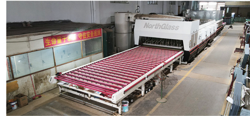
Flat and curved two-way tempering furnace 大型平弯双向钢化炉
